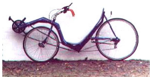
Figure 1 The complete rear-wheel support is from an old bicycle, as is the frontfork, the handlebar and various components
